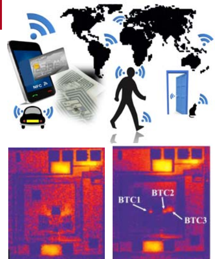
Fig.1) Above- Applications of Radio Frequency Identification Device (RFID). Bottom- Temperature Amplitude ( I_{S,IT} ) images of a RFID Device. From left to right the activation of different Integrated Circuit parts is assessed and quantified with a real time lock-in detection.
