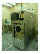
• A Sirius Semitool equipment for cleanings based on O<sub>3</sub> and hot water spray for CMOS compatible wafers up to 150mm
