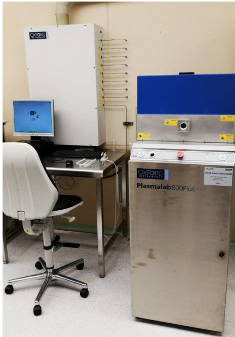
Oxford IPT, Plasmalab 800 Plus: 1 chamber, MNC (contaminated samples), Wafers up to 200 mm diameter or below.
