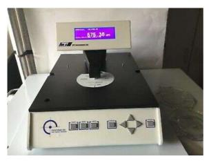
**Geometrical characterization: Proforma 300**Wafer Bow and Thickness capacitive measurement
