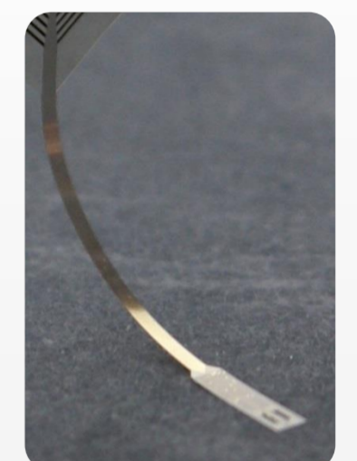
Flexible substrate technologies (SU8), devices of 25 \mu\text{m} width
